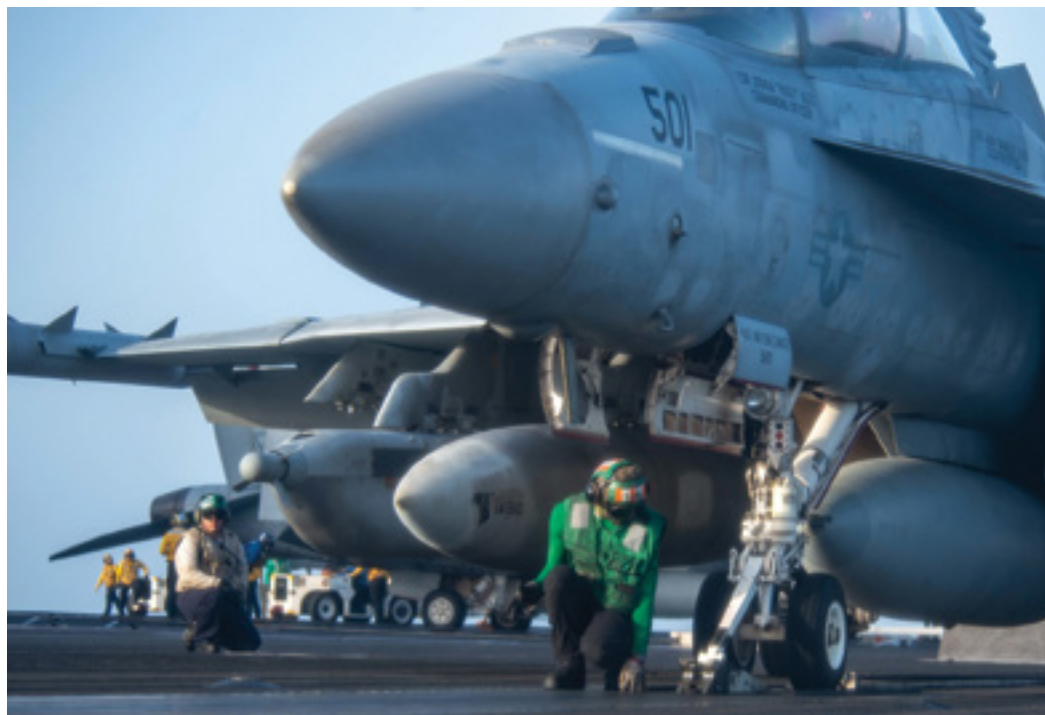
An EA-18G Growler electronic attack aircraft prepares to launch from the flight deck of aircraft carrier USS Ronald Reagan. (U.S. Navy photo)
