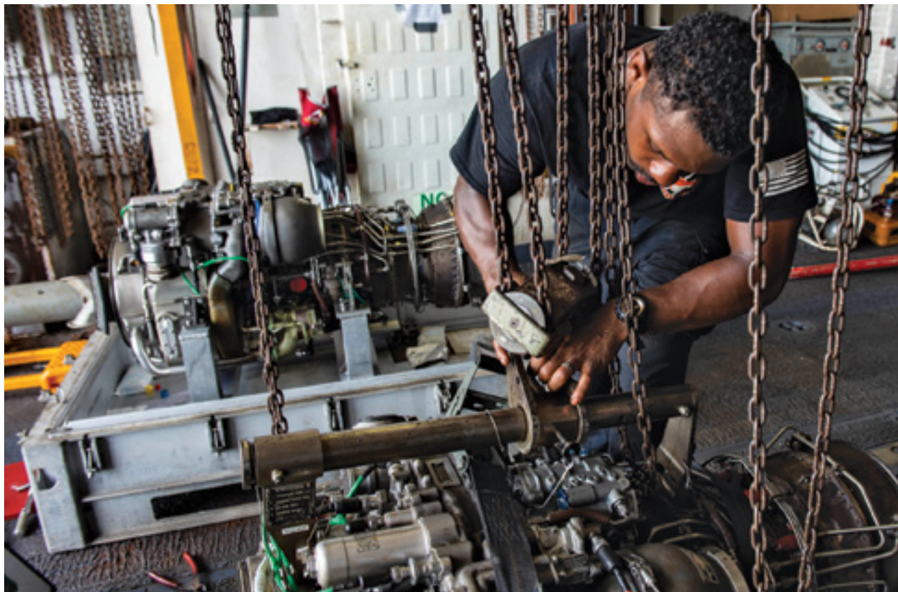
A U.S. Navy aircraft maintenance technician attaches a hoist to an MH-60R Sea Hawk engine aboard a guided-missile cruiser during operations in the Arabian Sea. (U.S. Navy photo)
