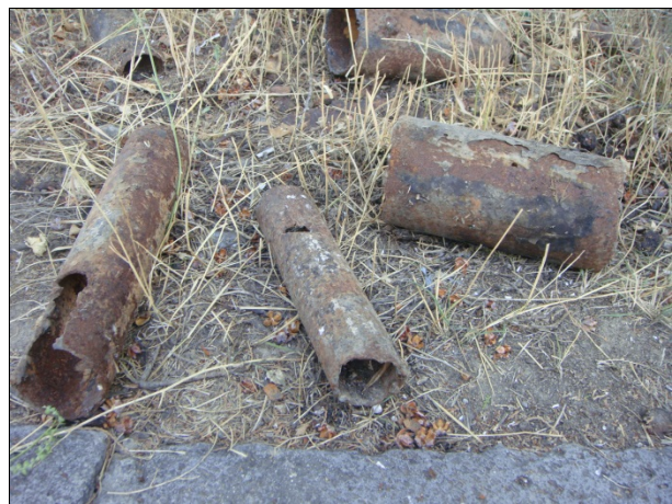
Some of the projects USAID funded under Task 2 included equipping a medical clinic with a solar air heating system (left) and replacing a village's corroded steel and cast-iron water pipes (right) with ones made of polyethylene. (Photos by OIG, October 2013)
