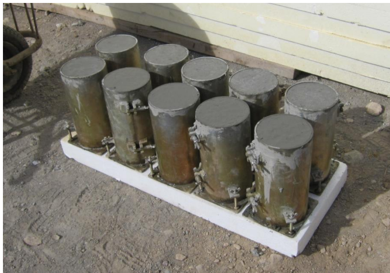
Concrete cylinders prepared at the Gardez 100-bed hospital site await compression strength tests. (Photo by OIG, November 2, 2010)
