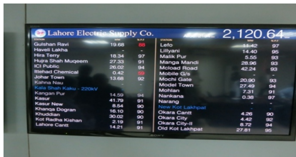
Under the Load Data Improvement Project, smart meters installed at the grid substation feeder panels (left) transmit real-time data about power distributed by Lahore Electric Supply Co. The data appear on screens in the company's newly established control center (right). (Photos by OIG, June 2013)
