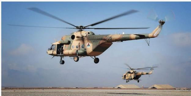
The SMW has received all 30 Mi-17 helicopters planned for delivery. The aircraft conducts light lift, personnel transport, CASEVAC, resupply, air interdiction, aerial escort, and armed overwatch missions. Every aircraft is armed with two 7.62mm door guns, and 12 have 23mm Forward Firing Cannons.
