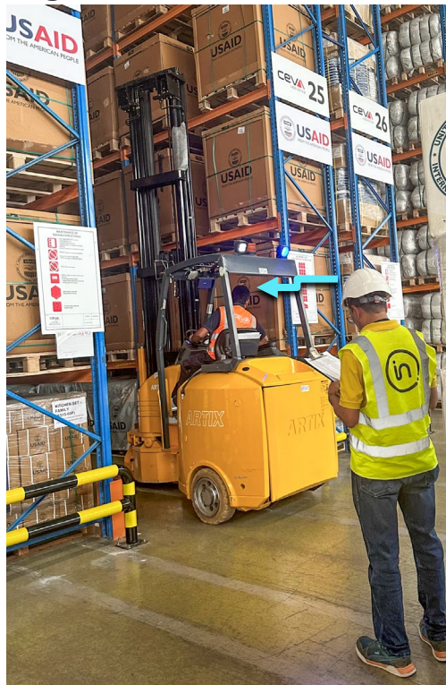
Left: A warehouse employee wearing an orange safety vest operates a forklift without a helmet in an aisle with USAID commodities stored on a six-shelf pallet rack 6 in the presence of an inspector wearing a helmet (see blue arrow).
