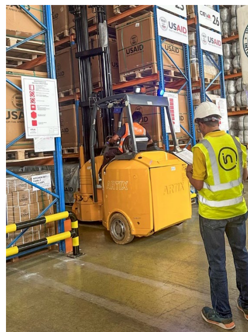
A warehouse employee without a helmet operates a forklift near a pallet rack with USAID commodities in the presence of a properly attired inspector.
